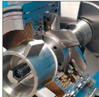
The 4-plate cutting system is driven by a step motor in combination with a PLC to guarantee always the optimal cutting point and therefore a constant product quality at a minimum of wear on the cutting tools.
